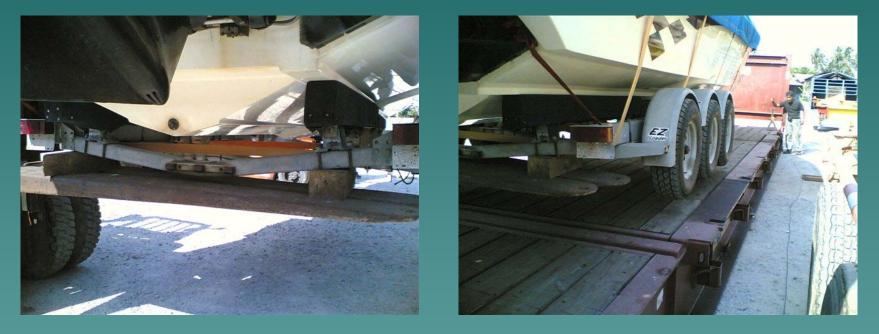
Note that the forks are positioned at the centre of gravity of the boat. It is also raised by 2 timber blocks to support the boat's trailer. If the boat is without trailer, a cradle has to be made to support the boat and a crane with sling and spreader bar to do the lifting.
